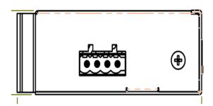
TEP 1 – Take out 4 pin terminal block located in the included mounting kit package.
