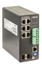
The series includes robust, high-quality switches for the implementation of powerful 10, 100 and 1000MBit/s Ethernet ring network structures according to IEEE802.x. All six copper ports feature Power over Ethernet with PoE and PoE+. These devices are specifically designed for video networking. The switch allows one or more fault-tolerant fiber optic rings to be built via two or more ports.
