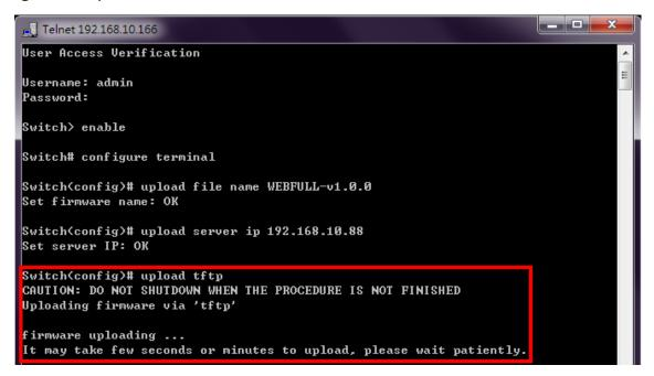
6. After uploading, the system will **verify** the uploaded file. If the verification passes, the new firmware file will be installed. Ensure the system is **powered on** and the system will **reboot** automatically after the firmware is completely installed.
