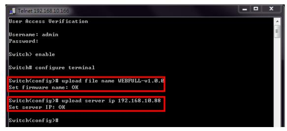
5. Start to upgrade the firmware file by specifying "upload tftp". The system starts to upload the assigned file by the TFTP. This takes a few minutes.
