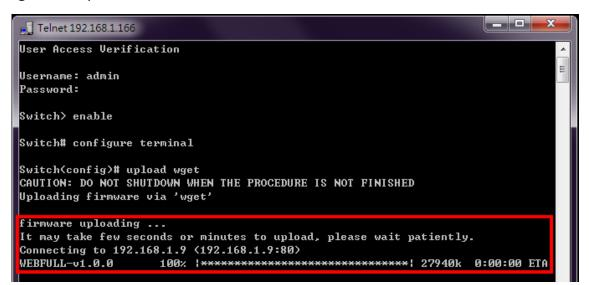
6. Once the uploading is complete, the system will verify the uploaded file. If the verification passes, the new firmware file will be installed. Ensure to keep the system powered on and the system will reboot automatically after the firmware is completely installed.
