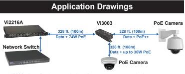
Vi3003 allows for the transmission of two cameras over a single camera run or adding a new camera close to an existing camera.
