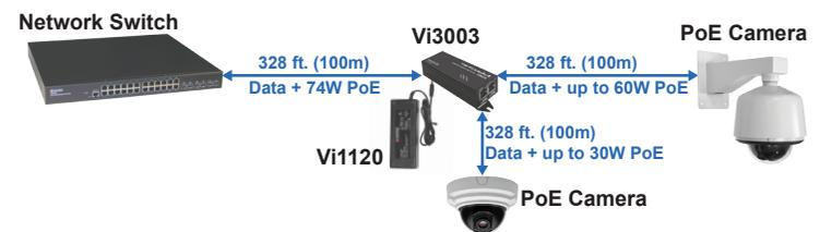
Vi3003 can provide over 60W PoE on port 2 and 30W PoE on port 3 using Vi1120 external power supply.
