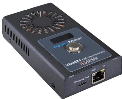
Vigatron's patent pending Vi00024 is an innovative test tool that installation reliability by measuring PoE capacity at any point of a networks before installing a camera. The Vi00024 simulates PoE devices and measures the maximum PoE capacity received from the PoE source over the network. It is compliant with IEEE 802.3af/at/bt standard up to 74W.
